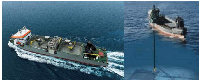
Figure 10.3-2 Scour Protection Installation via Fall Pipe with ROV-guided Lower End
