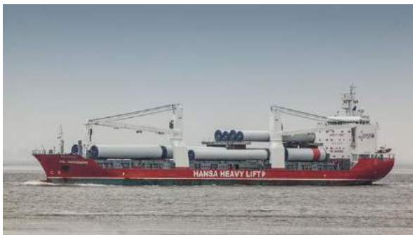
Figure 10.3-6 Multi-purpose / Heavylift Vessels with WTG Components
