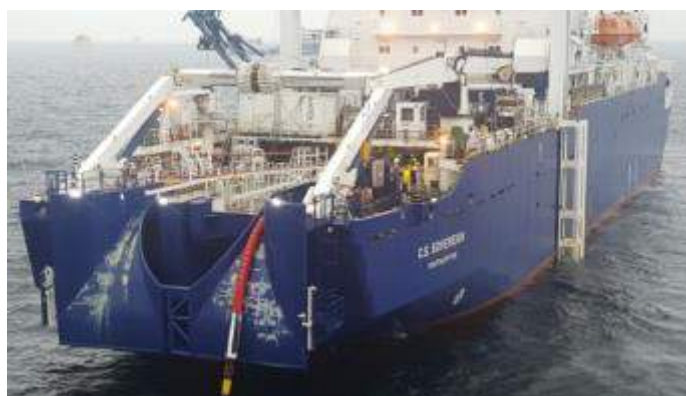
Figure 10.3-5 Inter-array Cable Installation Vessel
