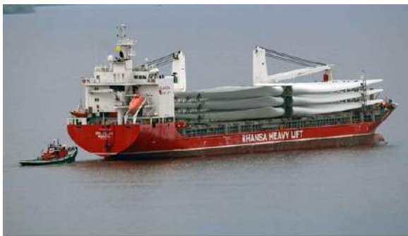
Figure 10.3-6 Multi-purpose / Heavylift Vessels with WTG Components
